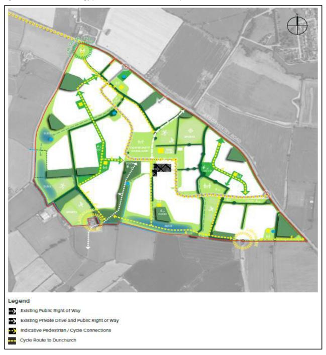
2.2.2 The southern roundabout would be constructed first to provide access to the Phase 1 of the development (circa 265 dwellings). The northern roundabout would be provided as part of Phase 2, with the employment access also coming forward in Phase 2 of development (dependent on demand).
